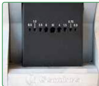
PNB-4KE detail of the crimping zone.
