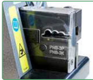
PNB-3P detail of the crimping zone.
