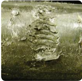
Minor cable damage caused by thread contact
