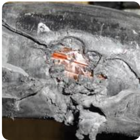
Major cable damage caused by thread contact
